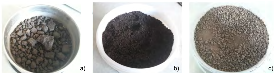
Figure 1: a) Non-passing fraction of the 5 mm sieve, b) sieved hydrocarbons polluted soil, c) depolluted soil
