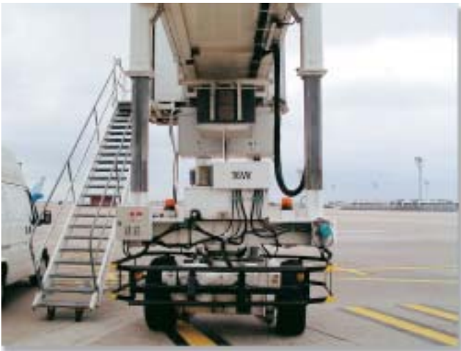
Drive unit of a boarding bridge
